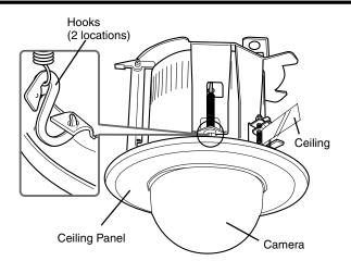
Attach the ceiling panel (supplied) to the 2 hooks on the Ceiling Recessed Bracket.
